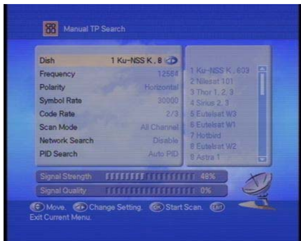
STEP 5 "Manual TP Search" Menu appears. Ignore the Dish name. Using down key scroll down to "Frequency"
