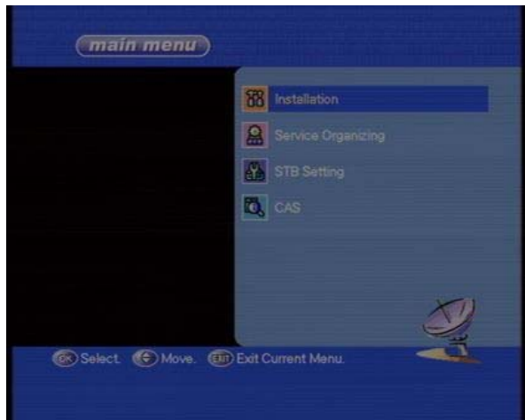
STEP 1 Using the Remote Control press "Menu" button. Main Menu screen appears with "Installation" highlighted
